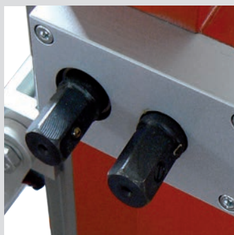
Dual speed motor carriage feed system
