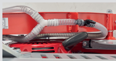
Double water inlet for improved blade cooling
