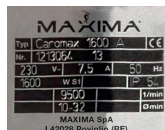
High speed motor: 9500 rpm
