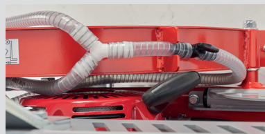
Double water inlet for improved blade cooling
